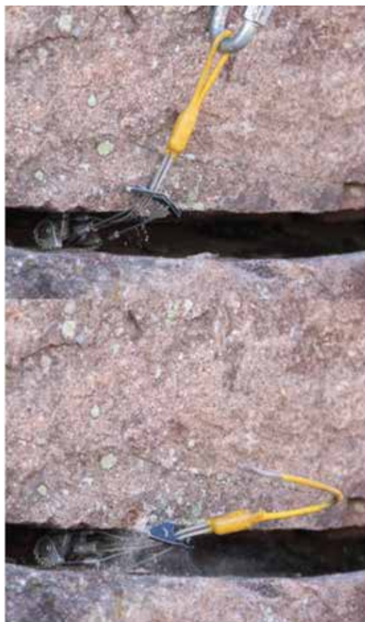
Figure 10. Failure mode of the cams.
