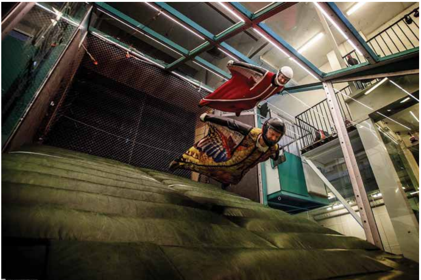
Figure 10. Wingsuit pilots training in an inclined wind tunnel (Stockholm, Sweden) having a variable inclination range that covers the stationary glide performance of current wingsuit models. Take-off and landing are from/to the floor, meaning that only Phase 4 can be realistically trained. Photo courtesy of Espen Fadnes and Håkan Nyberg.
