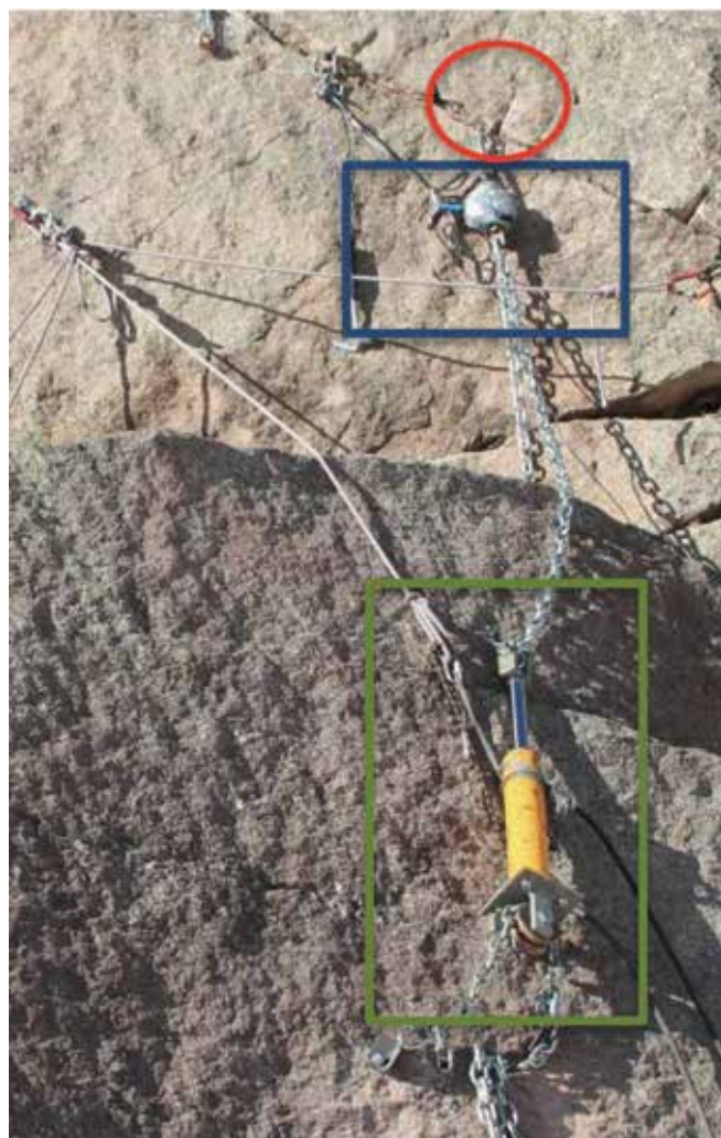
Figure 1. Extraction tests: the oleo-dynamic piston in the green box, a gauged uniaxial load cell (50 KN rated) in the blue box, the specimen placed inside the red circle.
